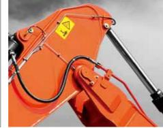
The adaptability to harsh dust work conditions has been improved by increasing the lubrication point of the arm connection unit.
