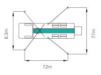
Front outrigger type X(Diagonal) Extension Rear outrigger type Swing-out
